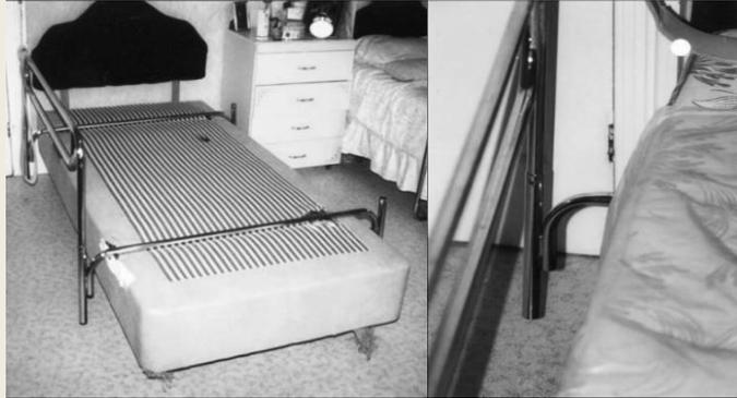
On inspection, the locking mechanism to secure the bed rails against the sides of the bed (under the mattress) was missing.
